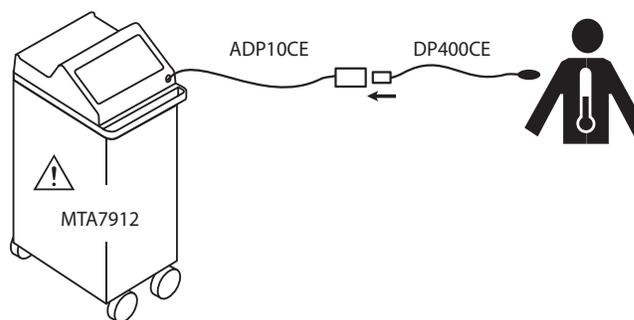
Figure 3—Disposable Probe/Reusable Adaptor Cable
