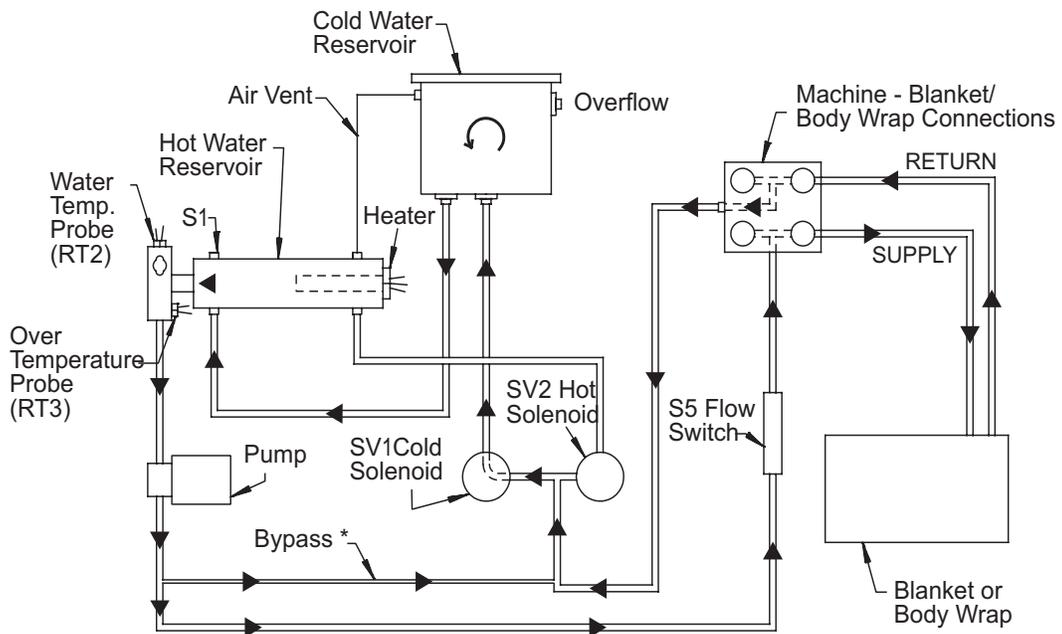
\*Water bypass prevents overheating when a blanket or body wrap is not connected to the Medi-Therm III.
