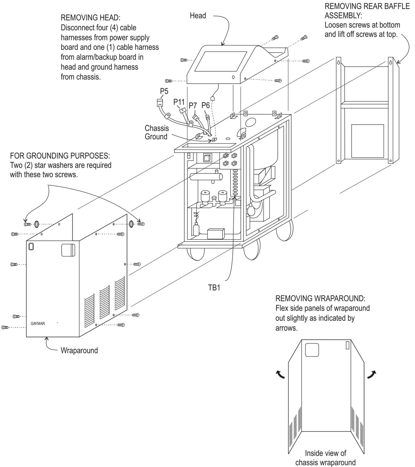
Figure 18—Machine disassembly
