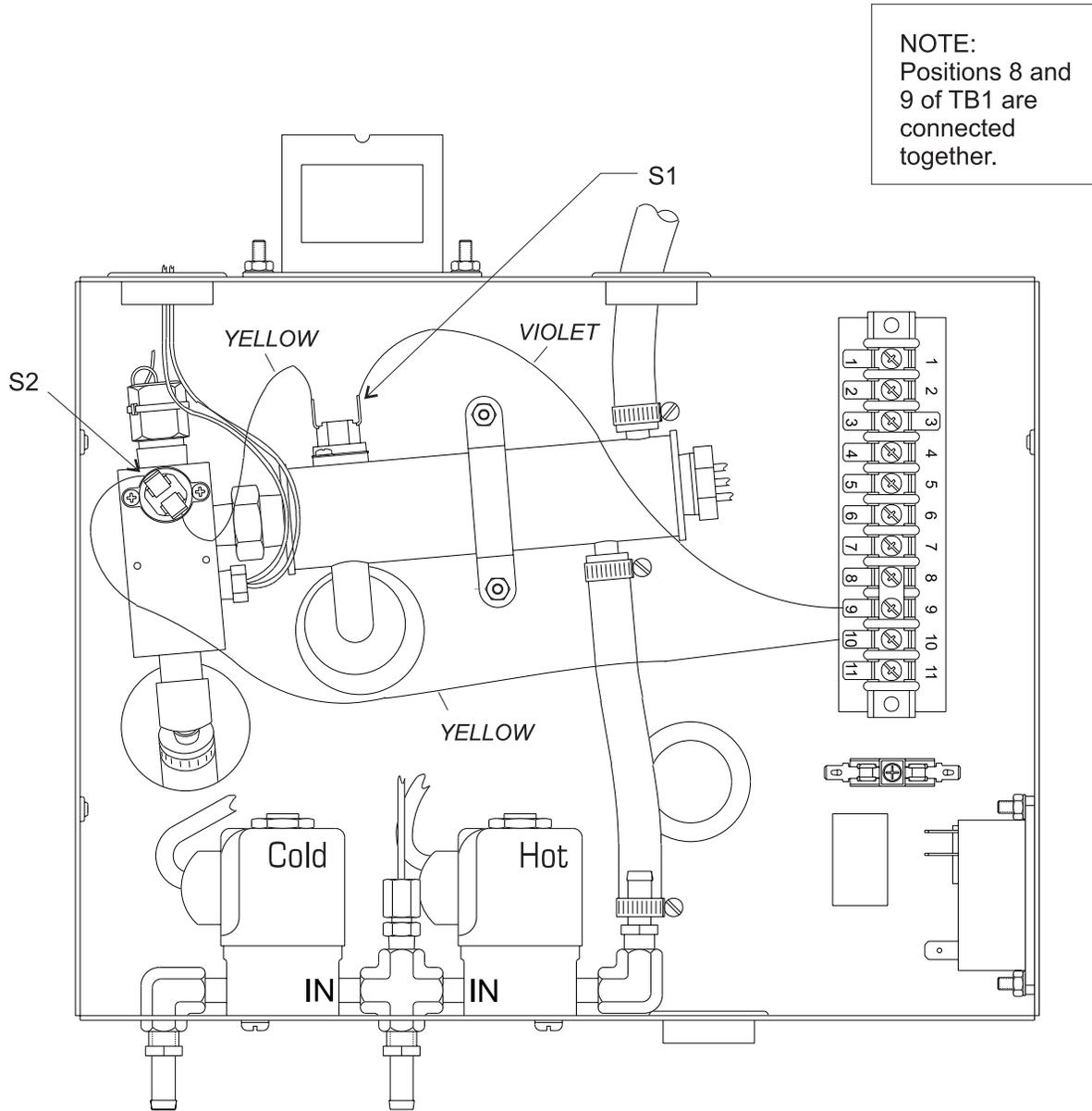
Figure 21—Thermostat Wiring Diagram
