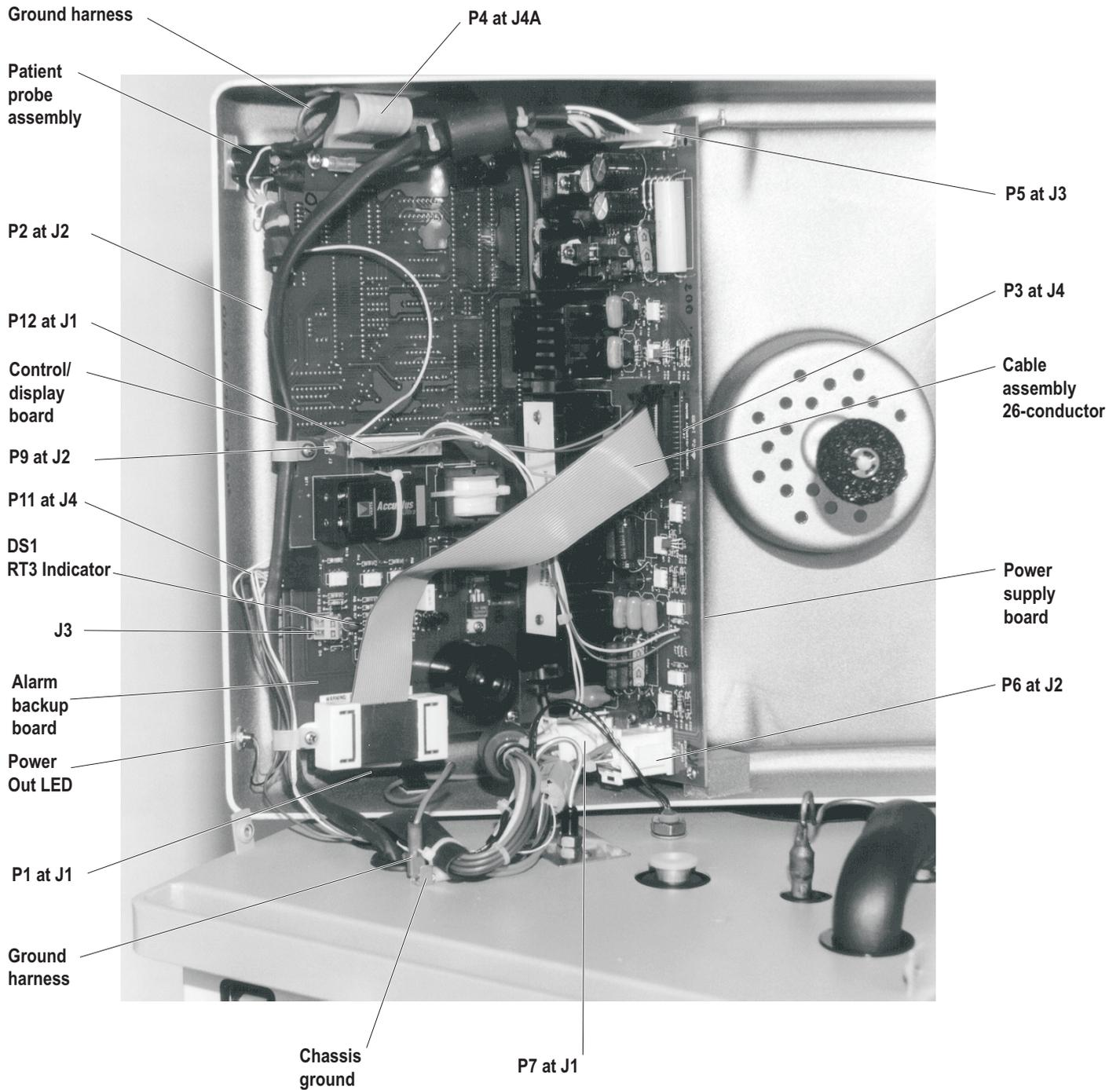
Figure 14—Circuit Boards and Connectors (head)
