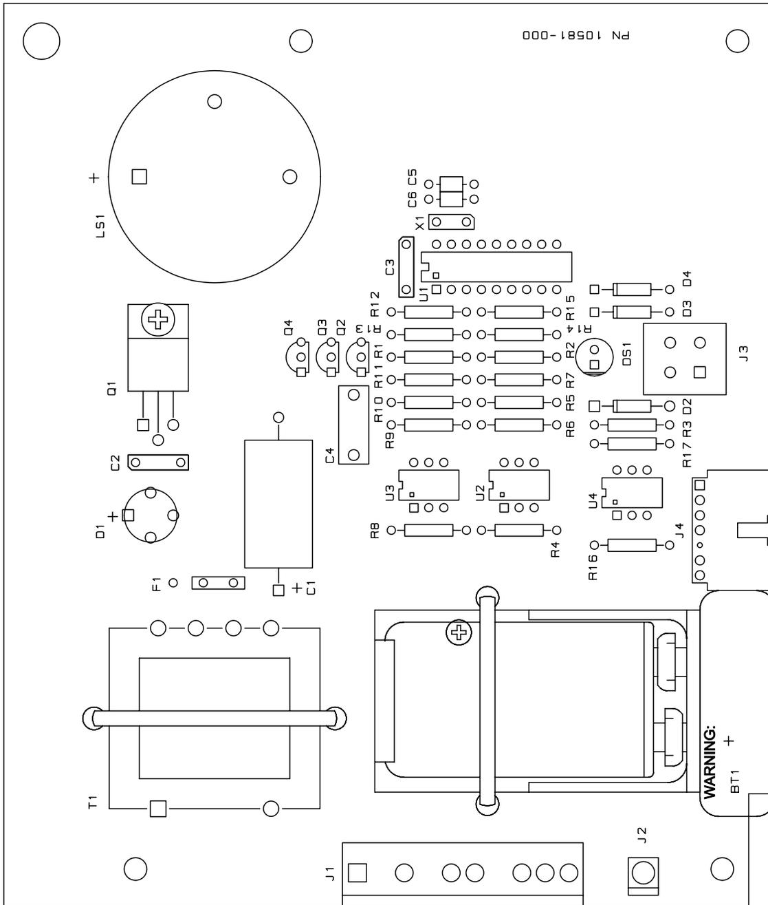
Figure 24—Alarm/Backup Board
