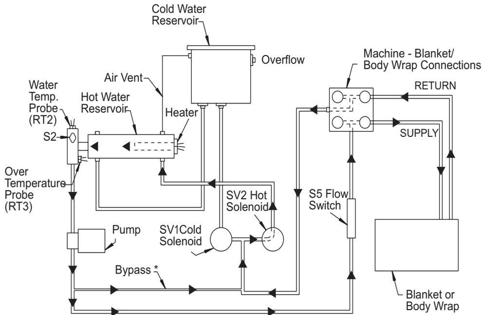
\*Water bypass prevents overheating when a blanket or body wrap is not connected to the Medi-Therm III.
