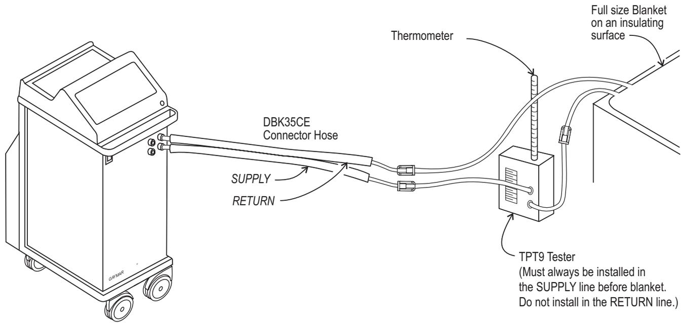
Figure 17A—Test setup [using TPT9 Tester and Thermometer]
