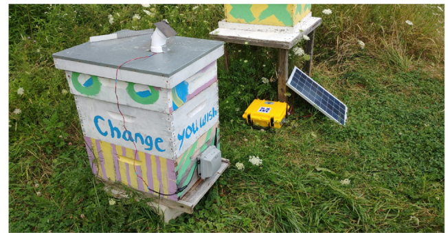
Fig. 2. A Prototype 3 beehive monitor unit is located just above the hive entrance. The base station is nearby, in a yellow weatherproof container. The two were powered by separate solar panels, one on top of the hive for the Doppler unit and for the adjacent base station. (For interpretation of the references to color in this figure legend, the reader is referred to the web version of this article.)
